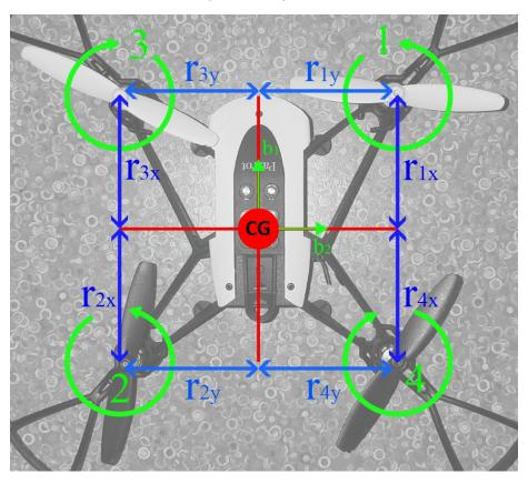
The diagram to the right represents the thrust, rotation, and the distance between the props and the CG (also referred to as *l* in the previous report, when looked at on the xz plane). Each motor/prop is numbered, 1 and 2 have the same rotation while 3 and 4 have the opposing. We can use this information to find some equations for the moment of pitch (L), roll (M), and yaw (N). The moment matrix for these would look like:
